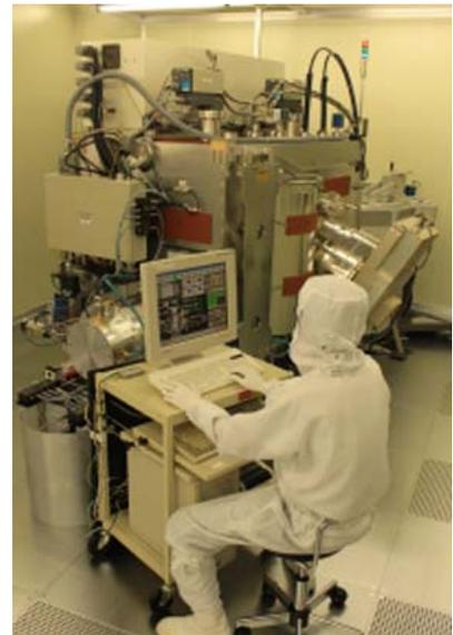
IBD (Ion Beam Deposition) system to form reflective Mo/Si multilayer for EUV lithography
