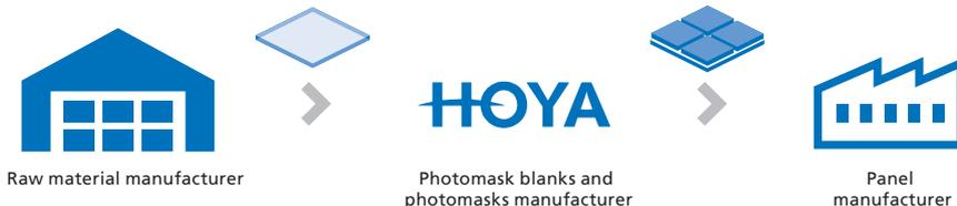
HOYA sources the substrate from raw materials manufacturers, and on that substrate performs polishing, deposition, and resist applications (blanks manufacturing). When the manufacture of the blanks is completed, HOYA conducts circuit pattern drawing, developing, etching, and resist stripping and cleaning, and delivers it to panel manufacturers (photomask manufacturing).
