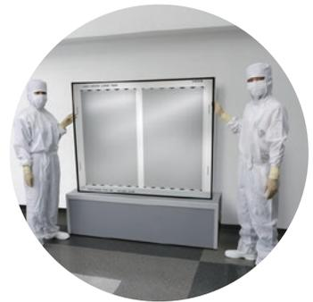
HOYA sources the substrate from raw materials manufacturers, and on that substrate performs polishing, deposition, and resist applications (blanks manufacturing). When the manufacture of the blanks is completed, HOYA conducts circuit pattern drawing, developing, etching, and resist stripping and cleaning, and delivers it to panel manufacturers (photomask manufacturing).
