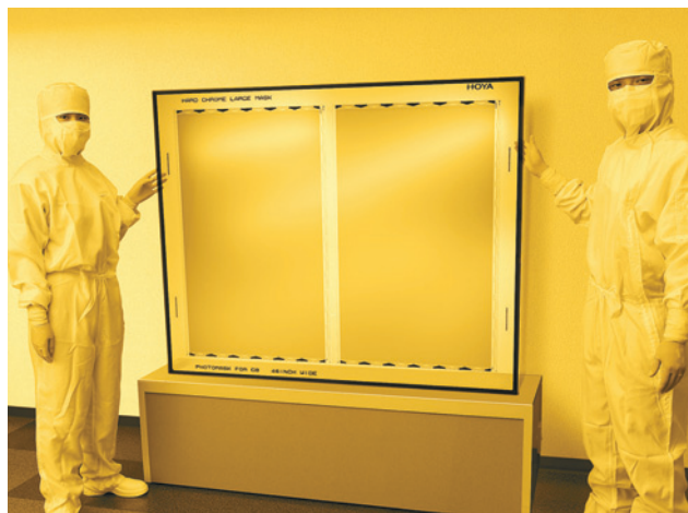
Large-sized LCD photomask (1,220 mm × 1,400 mm) used for eighth-generation LCD panels
