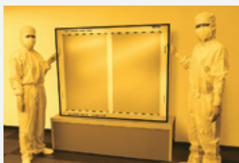
8th generation photomasks (1,220mm X 1,400mm) An 8th generation glass substrate can yield screens for six 50-inch LCD TV panels.
