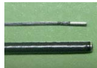
Upper: microfiberscope with an external diameter of 0.8mm. lower: FNL-7RP3, existing product with smallest diameter (Φ2.4mm at the tip of rigid part)
